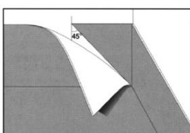
The corner seam shall be placed on one of the walls at a 45-degree angle.
