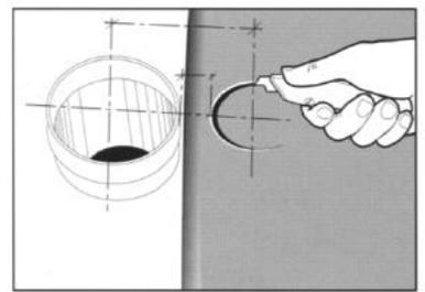
Around drain pipes, fold the sheet against the pipe and mark a line on the material where the center of the pipe is. Cut a hole about 25 mm (about 1 in.) smaller than the diameter of the pipe. As shown, cut the hole at the start of the fold. Heat the sheet vinyl and press it over the pipe. trim off excess material with a hook knife so that the break in the pipe wall is cleared.
