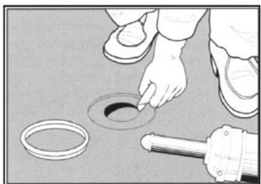
Around flush drain openings, heat the sheet and mark the location of the drain using a clamp ring. Then cut a small hole in the center of the drain within the mark. Heat the flooring and press the clamp ring down into the edge of the drain. When using an adjustable clamp ring, make sure it fits tightly. Trim the material around the perimeter of the ring.
